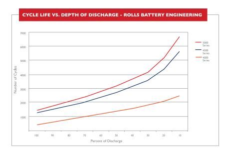
With traditional off-grid Renewable Energy systems, DOD is set to operate between 20% and 50% to maximize the life of the batteries. Battery-based systems are designed to allow a maximum 50% DOD as this offers a balance between capacity vs. cycle life, also taking into consideration the cost of replacement.
