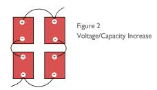
To increase capacity and voltage, connect the batteries in series parallel as shown in Figure 2.
