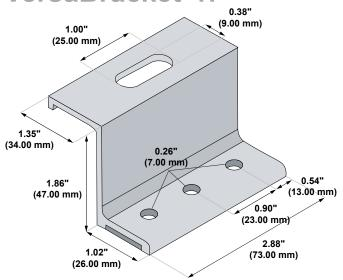
3 holes are provided for versatility. Some installations require only 2 fasteners. See the load table on the S-5I website and the installation instructions for more details.
