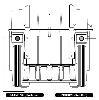
Figure 2-4 High Power 12-volt DC Terminals
