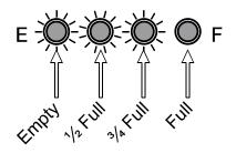
Figure 2-2 Battery level Indicator
