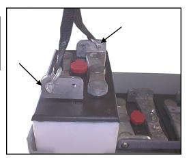
**Step 5** Connect the cell lifting strap into the holes of the terminals that are inline with the round post that protrude from the case. (see photo below) Lift the cells out of the tray. The first cell out of the tray will be harder than the remaining cells. If you find the first cell very hard to remove try another cell or lubricate with soapy water. If the clevis on the cell lifting strap will not slide over the terminal, slightly spread the clevis.
